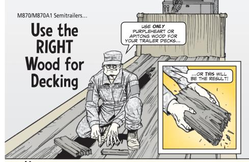
**M**echanics, when the wood decking in your M870/A1 semitrailer cracks and buckles, don't replace it with unapproved wood or rubber/composite products.
